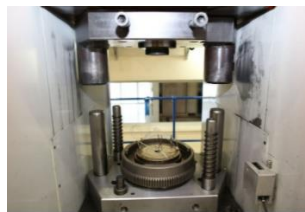
Figure 21. Mawi Mawi Crank press internal mechanism
